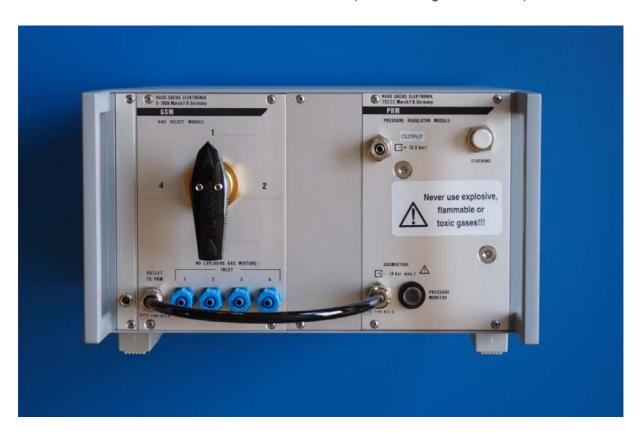
The Pressure Regulator Module PRM is a PLUGSYS module with a build in pressure regulator. The internal Pressure Regulator is set to regulate the output pressure to 0.5bar (7.2psi)
