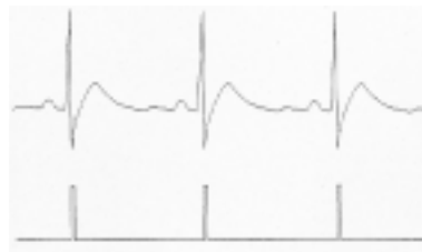
R-wave triggering with positive TTL pulses.
