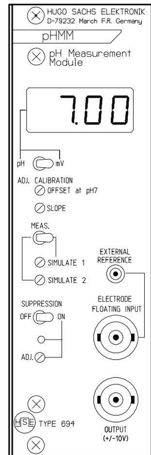
Fig. 1 Front panel
