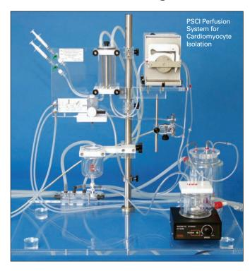
The Perfusion System for Cell Isolation (PSCI) is designed for harvesting individual cells from isolated organs such as mouse, rat or guinea pig heart, liver and other organs.
