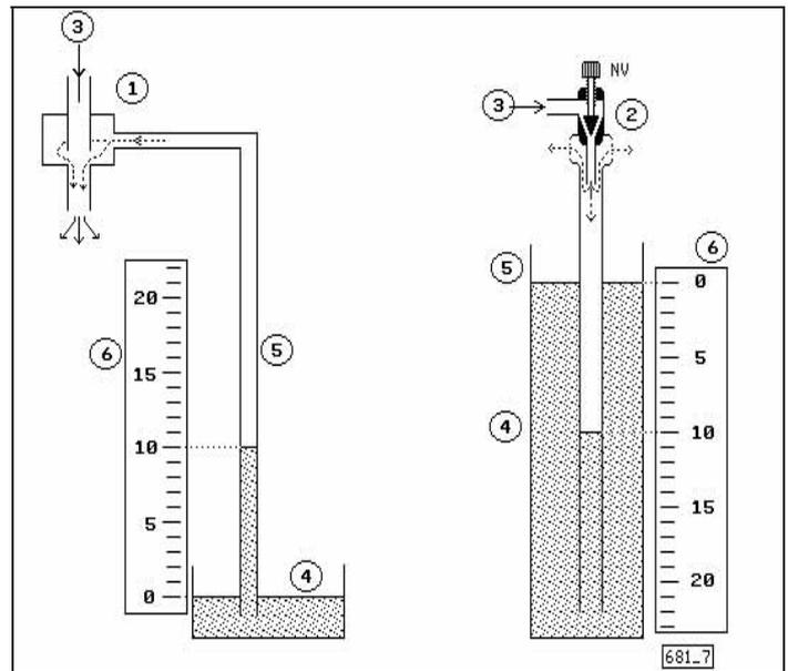
**Fig. 8:** Preliminary adjustment of the ventilation pressure using a simple water manometer.
