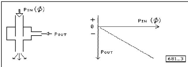
**Fig. 4:** Characteristic of the venturi nozzle
