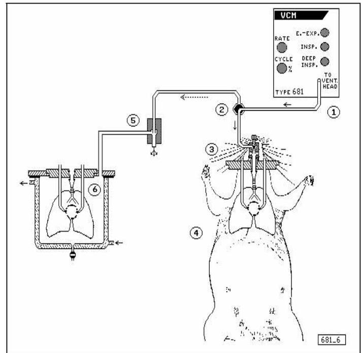
**Fig. 7:** Positive and negative pressure ventilation with the VCM
