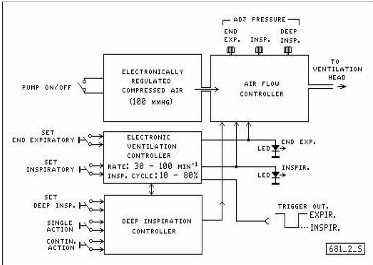
**Fig. 3:** Functional diagram of the VCM
