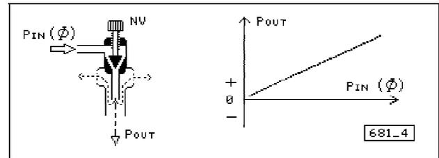
**Fig. 5:** Characteristic of the restrictor nozzle
