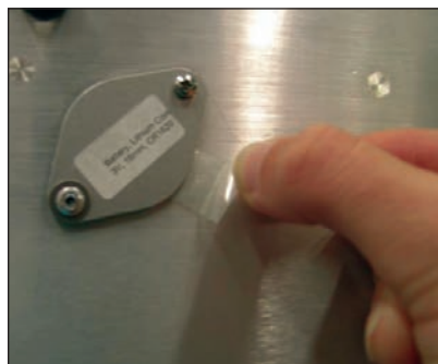
Figure 3: Battery Insulator must be removed before use.
