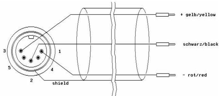
**Fig. 5:** Input socket for 3-pin plug
