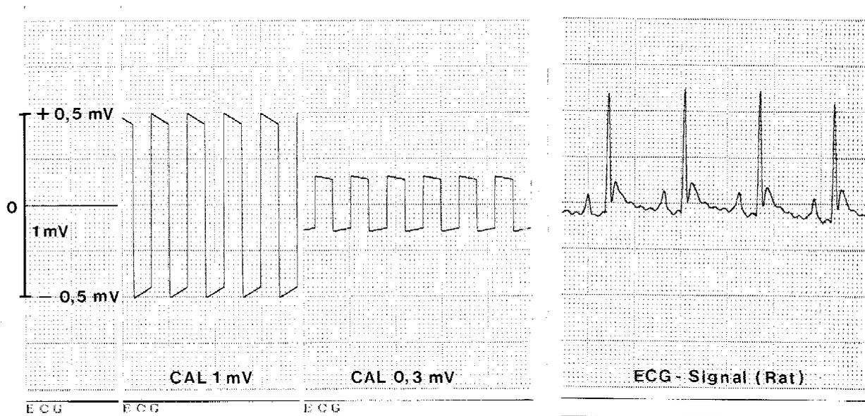
**Fig. 3:** Setting up an ECG scale on the chart, selected range  $\pm 1$  mV, see text above.
