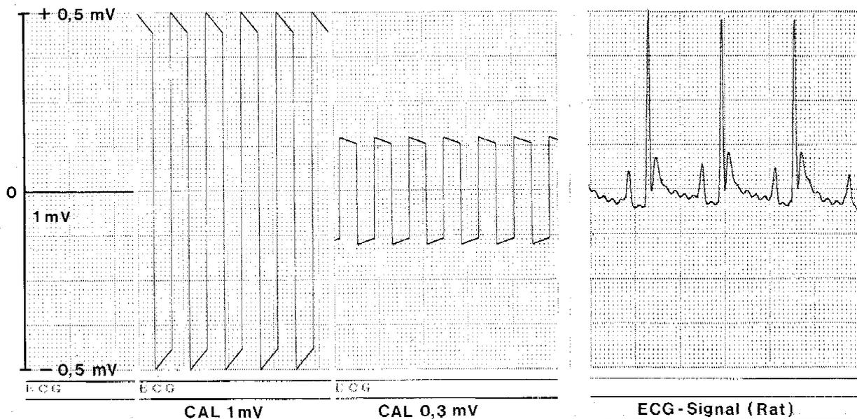
**Fig. 4:** Setting up an ECG scale on the chart, selected range  $\pm 0.5$  mV, see text above.
