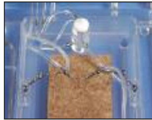
Mini ball joint holders support arterial and venous cannulae for rat liver perfusion
