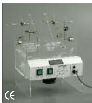
Basic Double Tissue Bath Set with 50-0652 Complete Simple Lever Assembly*
