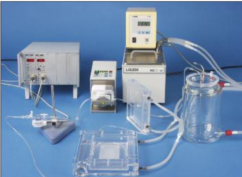
Moist chamber with peristaltic pump, SCP perfusion control system, perfusate reservoir and thermocirculator. Used for constant pressure perfusion for organs such as kidney and pancreas. The SCP perfusion control system includes flow measurement capability. By disabling the pressure control, the system can also work as constant flow perfusion system with pressure measurement.
