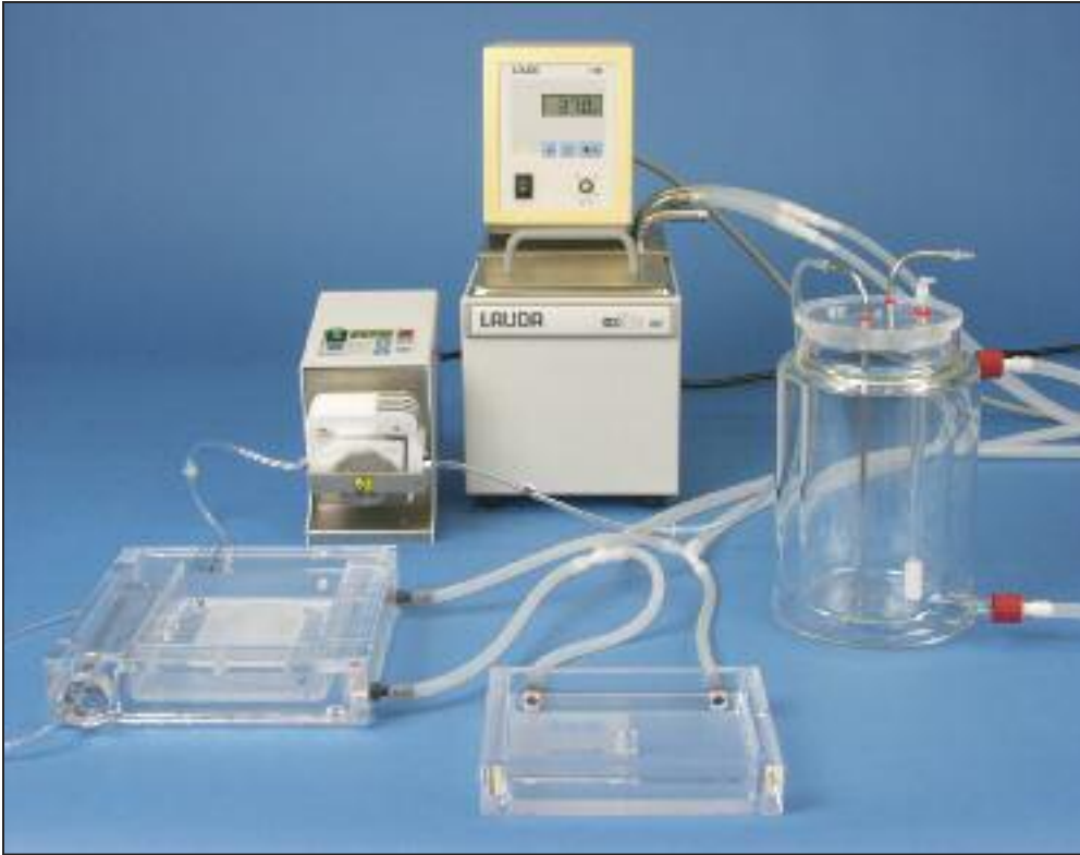
Moist chamber with peristaltic pump, perfusate reservoir and thermocirculator. Used for constant flow perfusion for organs such as Liver.
